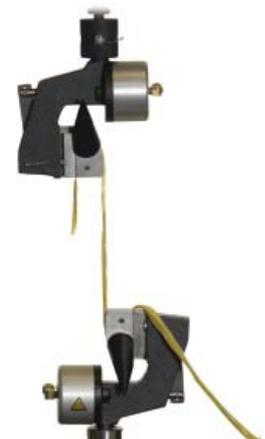
▲ Textile test using cord and yarn pneumatic grips
