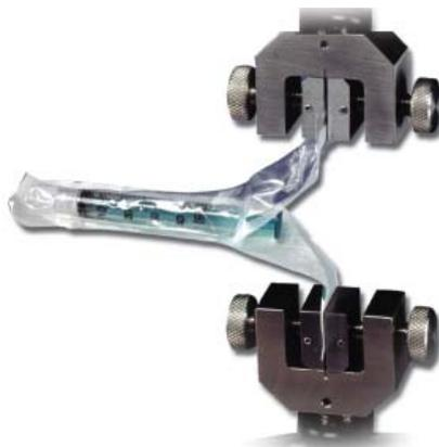
▲ Peel test using screw action grips
