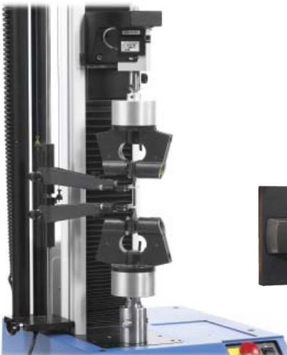
▲ Rubber test using long travel extensometer
