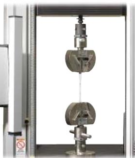
▲ Plastic test using Standard Video Extensometer (SVE)
